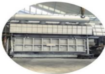
120T双室熔炼炉 120T double-chamber smelting furnace
